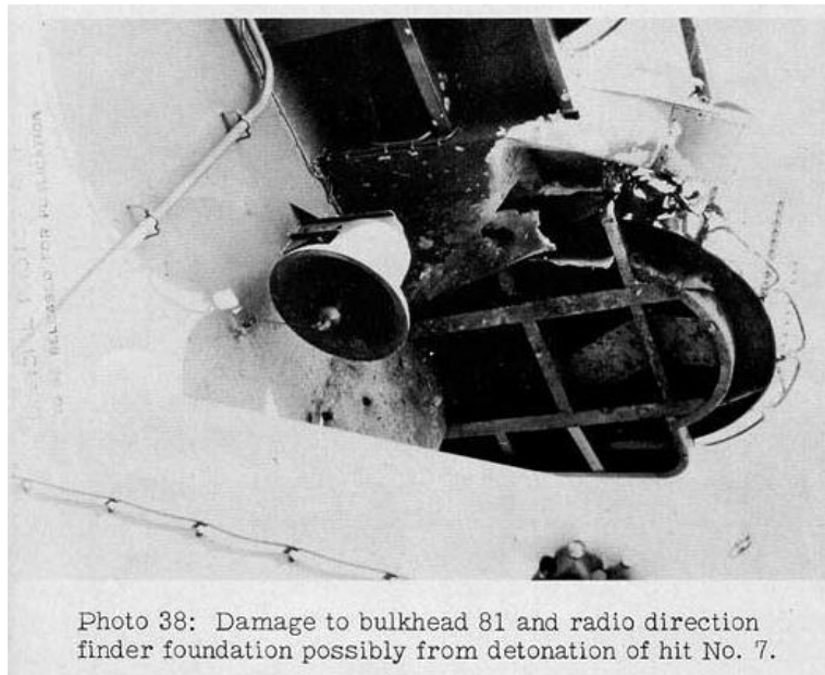
Figure 24 – Hit 7 – Shrapnel Damage near ship's bell
