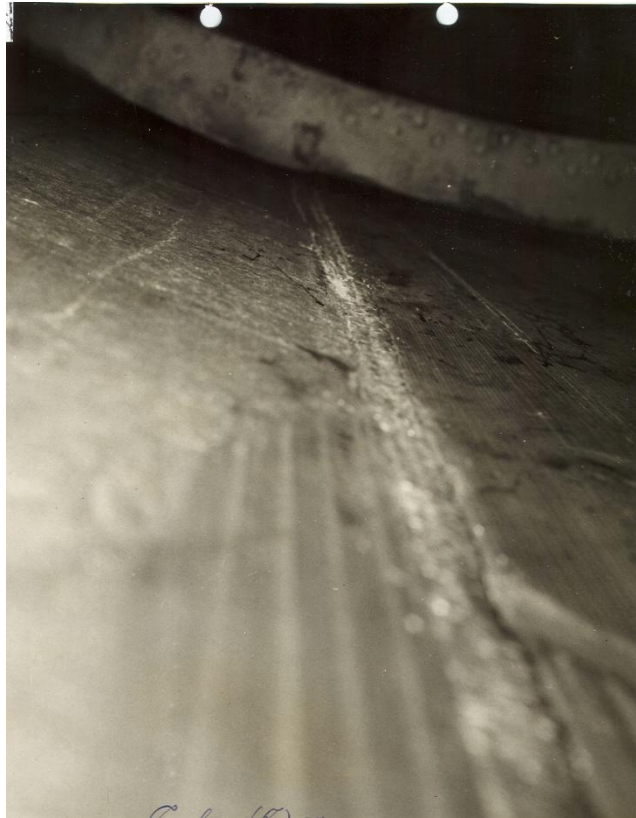
Figure 104 – Hit 26 – Damage to Roller Path
