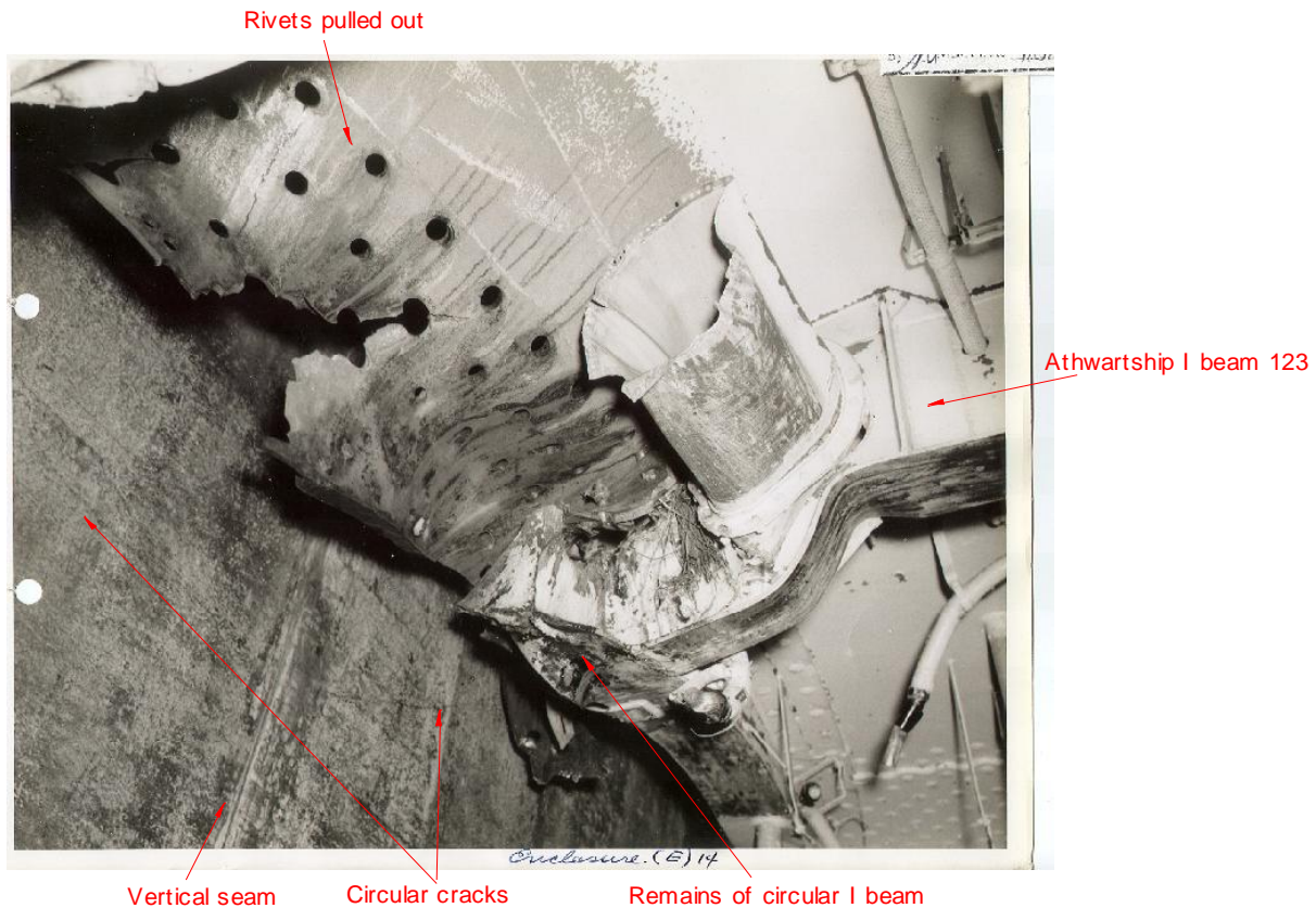
Figure 93 – Hit 26 – Remains of Circular I-beam
