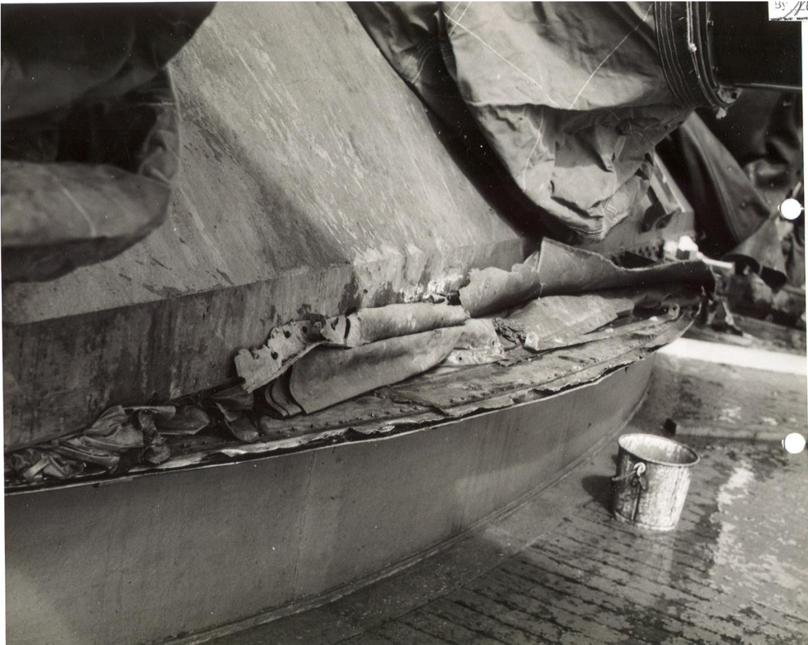
Figure 87 – Hit 26 – Damage to Turret Face
