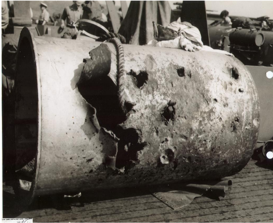
Figure 88 – Hit 26 – Damage to right gun sleeve
