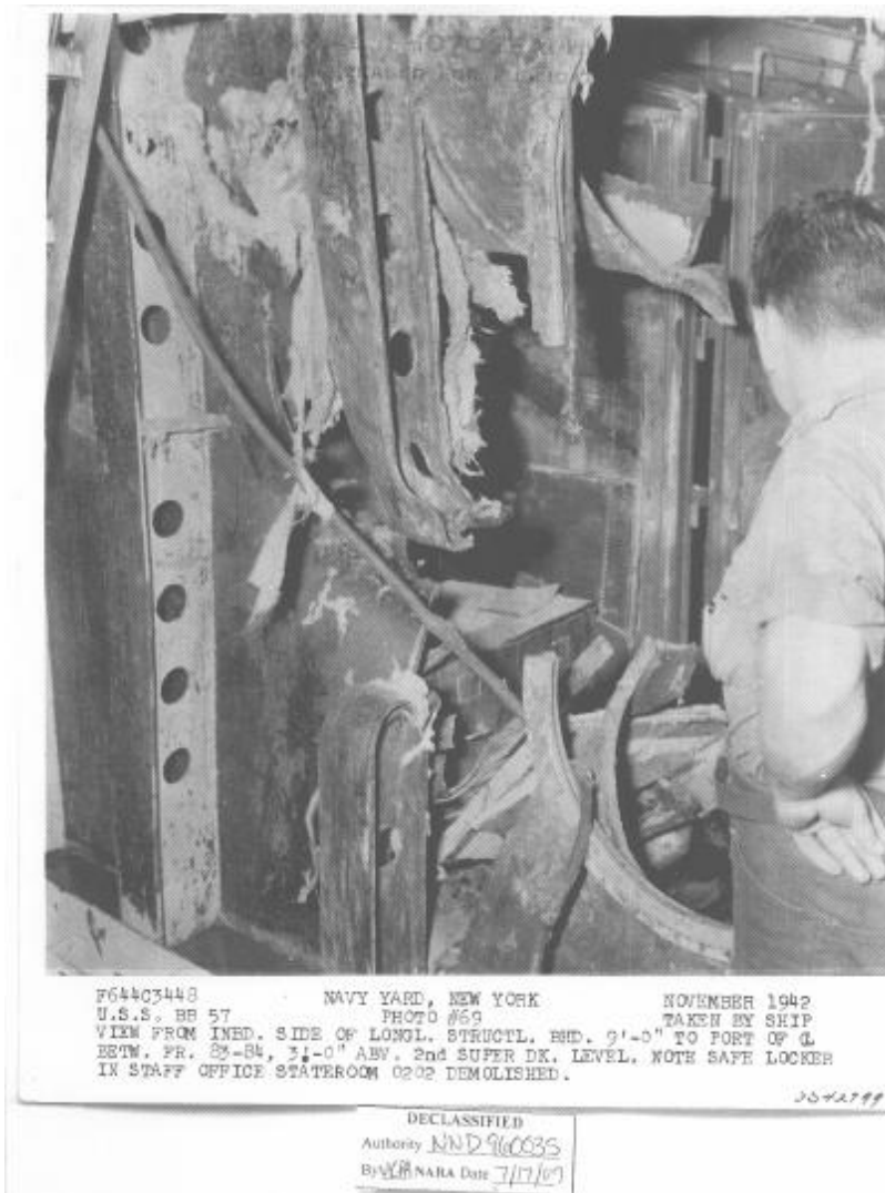
Figure 57 – Hit 17 – Damage to Internal Bulkhead of Staff State Room – View A
