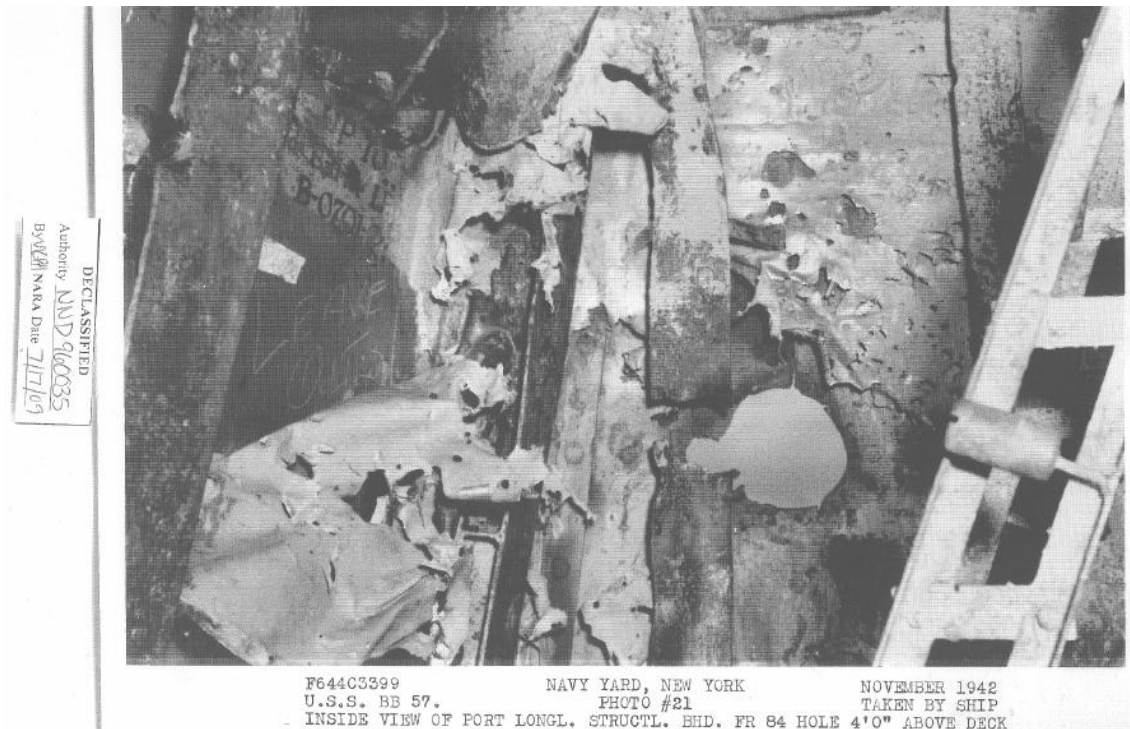
Figure 47 – Hits 13, 14 and 15 – Internal Damage – View C
