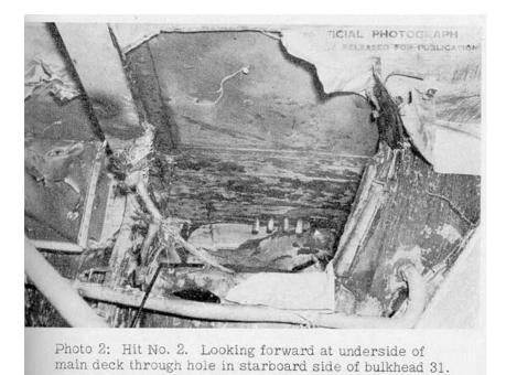
Figure 9 – Hit 2 – Interior Damage
